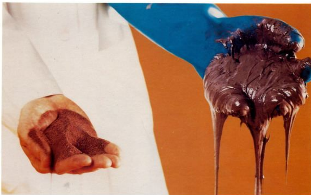
Haden Environmental Corporation operates the DryPure System to convert wet, sticky, paint often containing noxious substances into dry re-usable powder.
