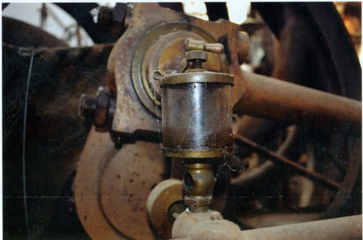
Oilers were used to lubricate bearings in machinery.
