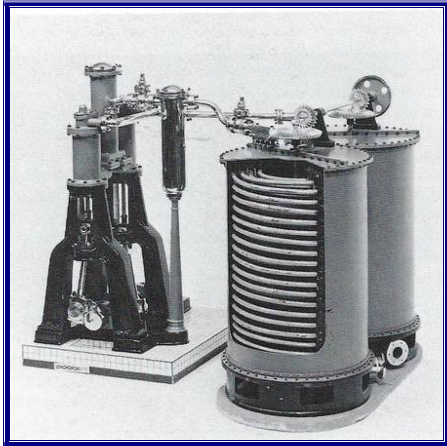
Model of Linde's first ammonia refrigerating system which had been installed in a Brewery in Trieste in 1877
