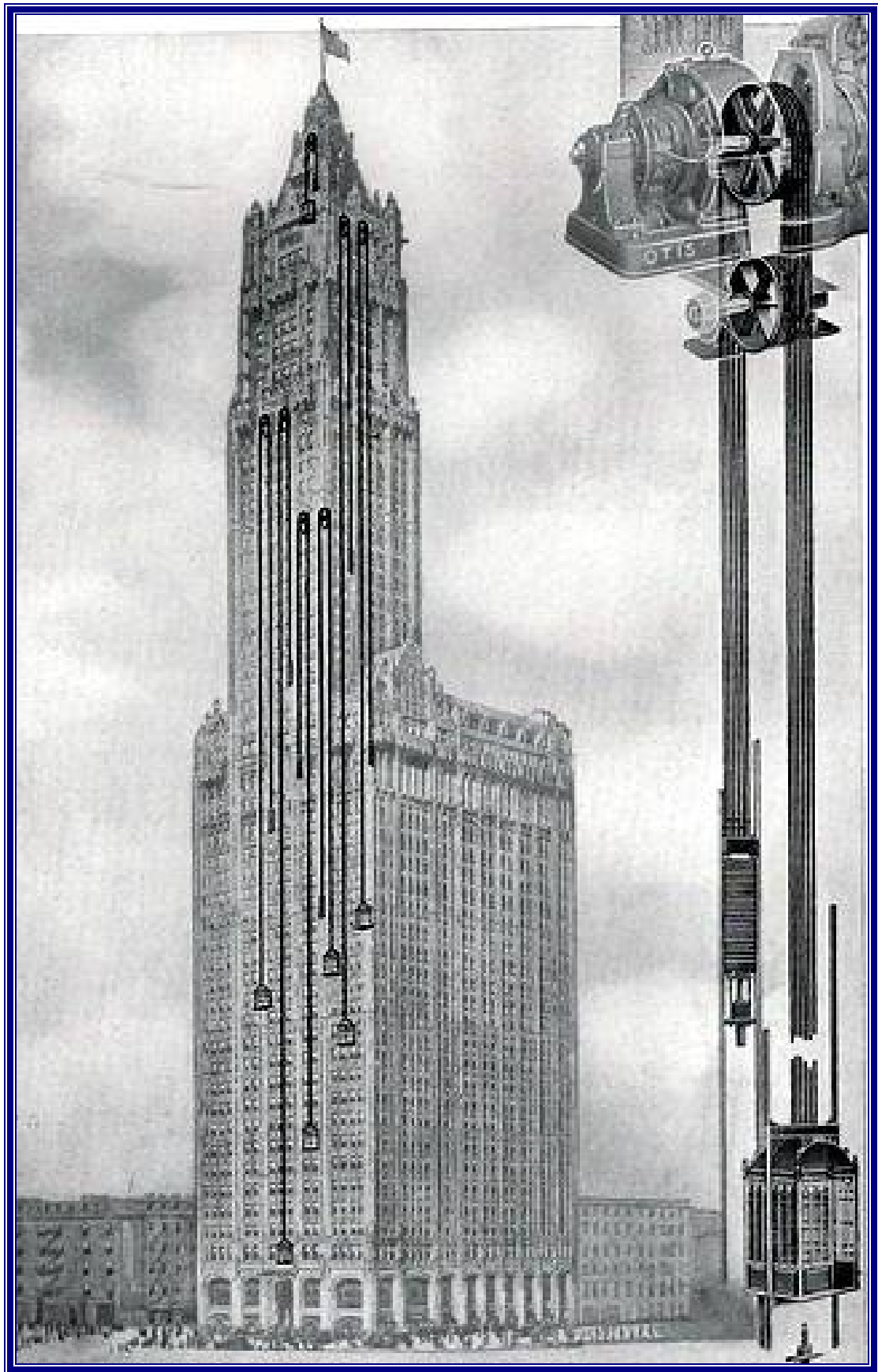
Diagram showing the six main Otis tower elevators, each with a speed of 700 ft/minute when loaded to 2500 pounds, then the fastest electric passenger elevators in the world
