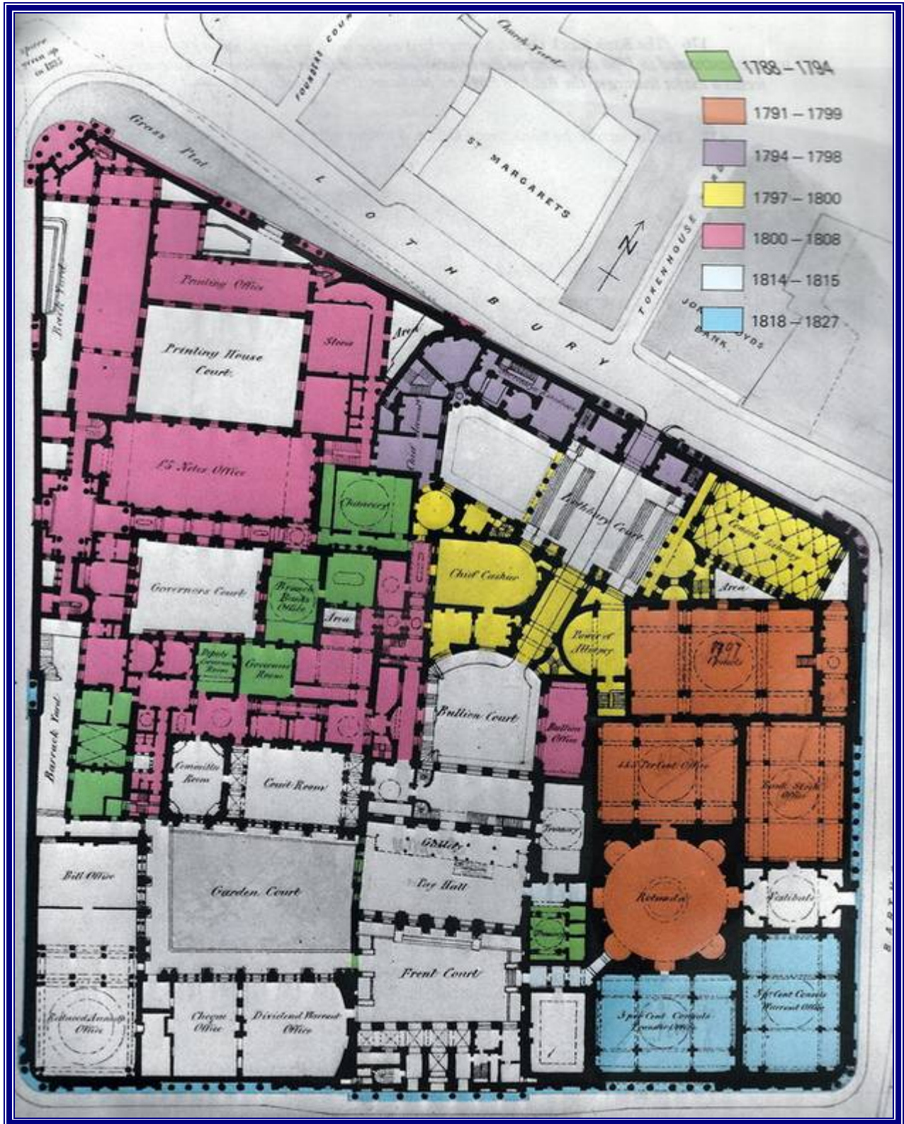
The Bank of England: Alterations and Additions, 1788-1827 during the time Soane was the architect. The Bank is popularly nicknamed "the Old Lady of Threadneedle Street."
