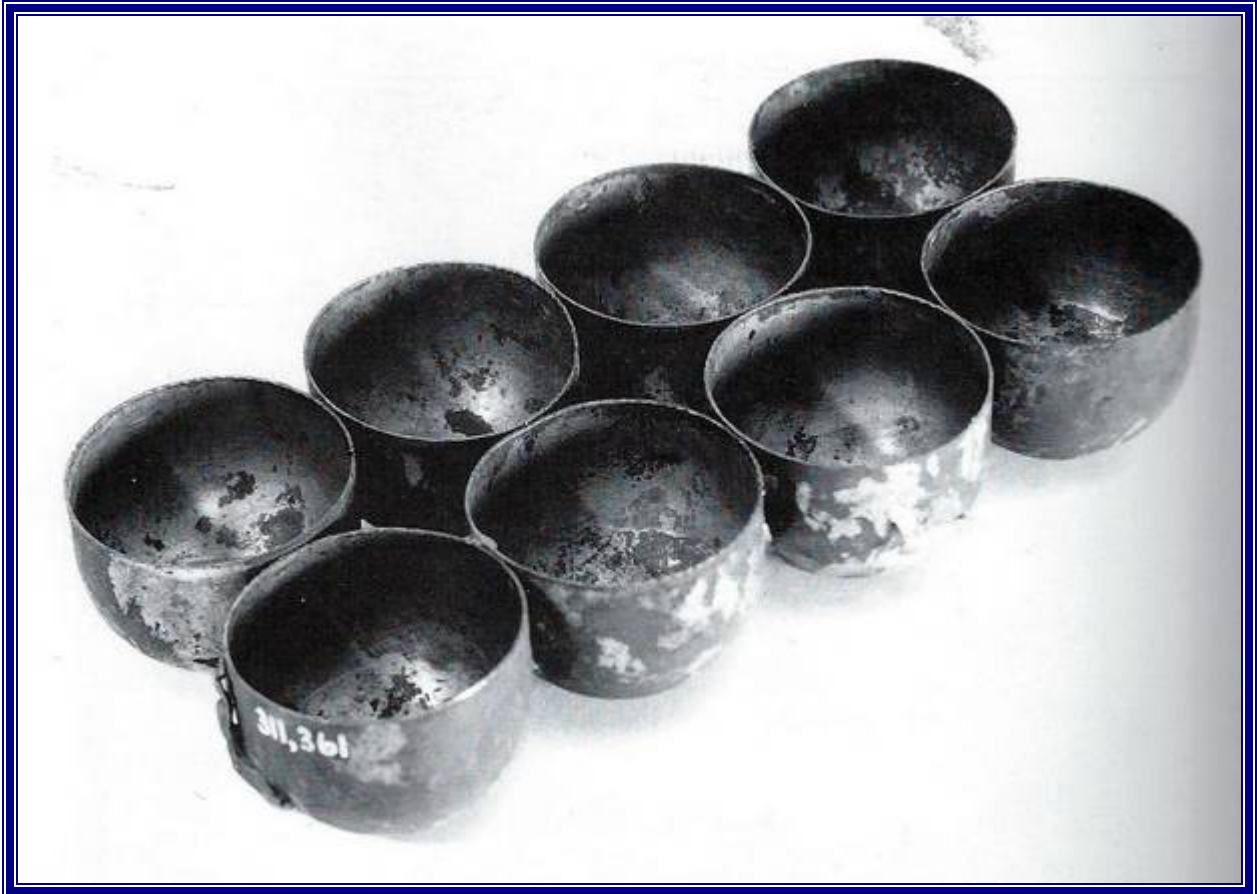
The ice-cube tray of the DOMELRE (based on muffin baking tins): Smithsonian Institution
