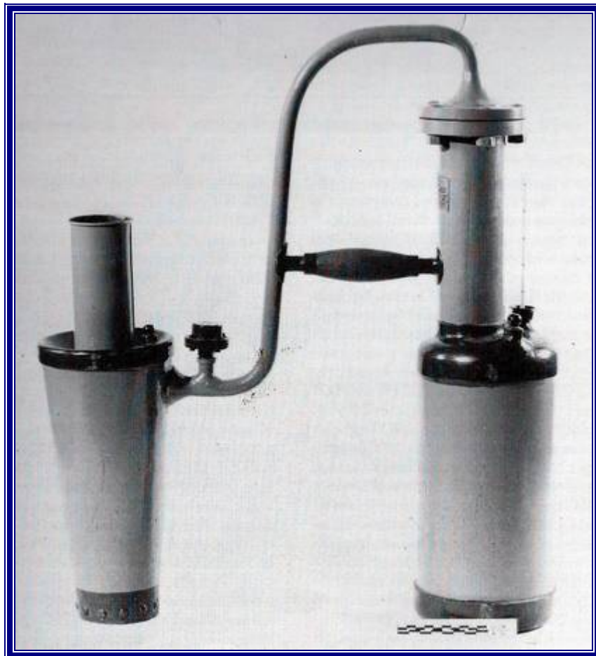
Carre absorption device (Smithsonian Institution, Division of Engineering & Industry)
