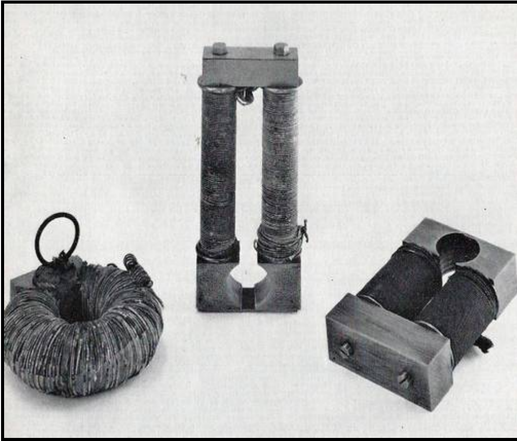
Experimental dynamo field models used by Hopkinson in his redesign of Edison's machine
