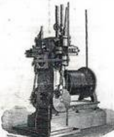
Relief Hoisting Engine. Cut G. Old Patent Non-revolving Screw Hoisting Engine, adapted for use in connection with Safety Platform, also especially fitted and readily adapted for working the ordinary screw-hoisting Machine, giving 90 feet per minute motion of Platform.
