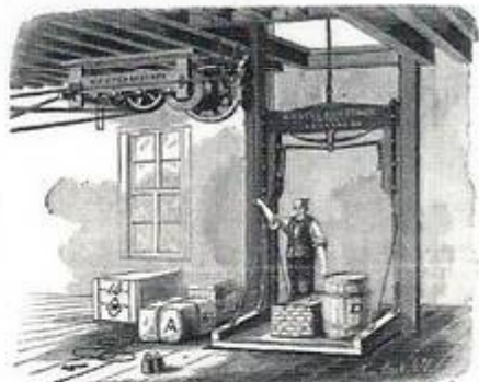
Universal Hoisting Machine. Cut H. Old Patent Lifting Power, Safety Platform and connection, for Factories, Mills, Shops, Bakeries, and all general business purposes where steam, water or gas power is at constant use. Motion of Platform 50 feet per minute.
