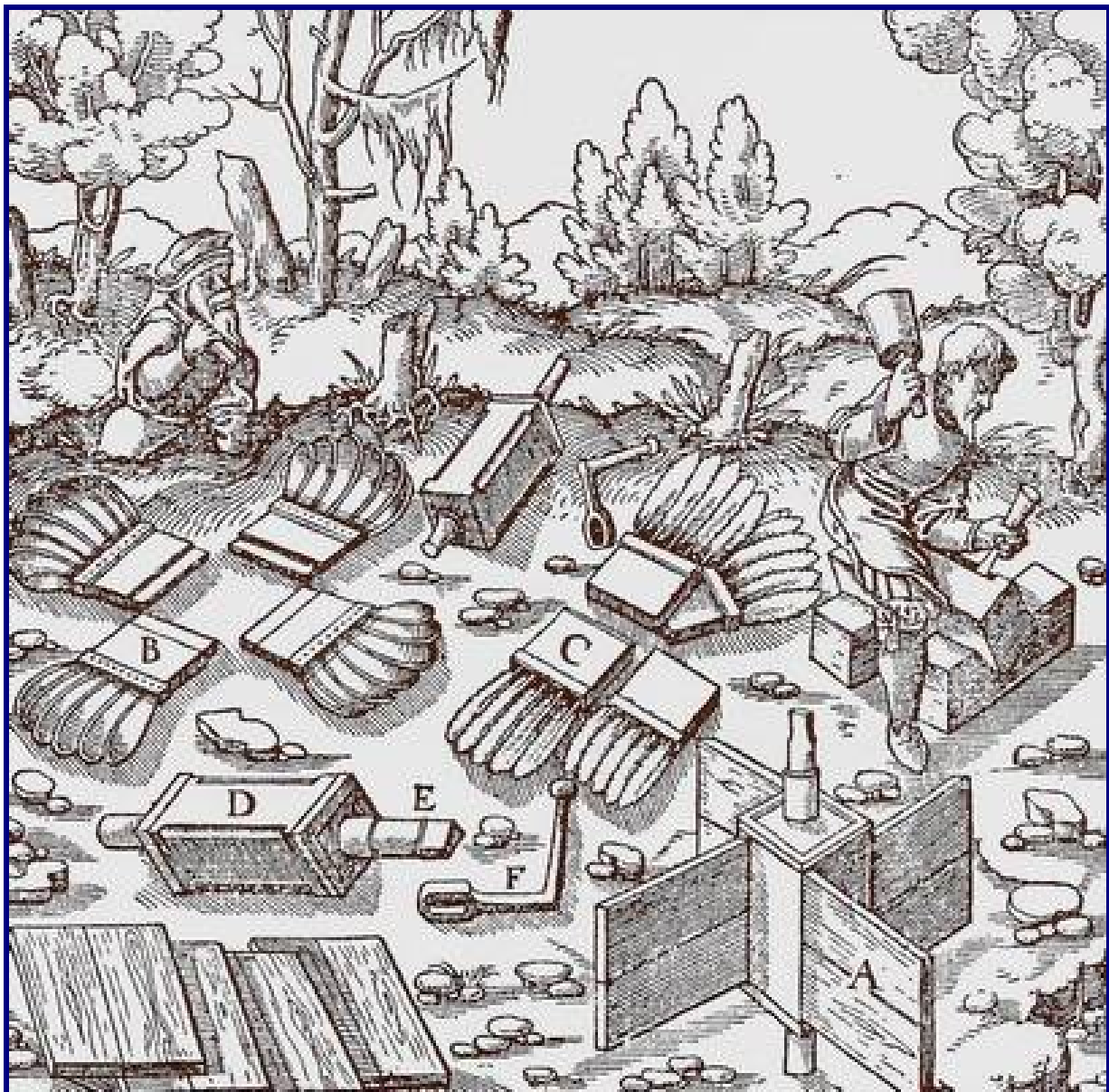
Making fans for mine ventilation, 1556, using fan blades tipped with goose feathers
