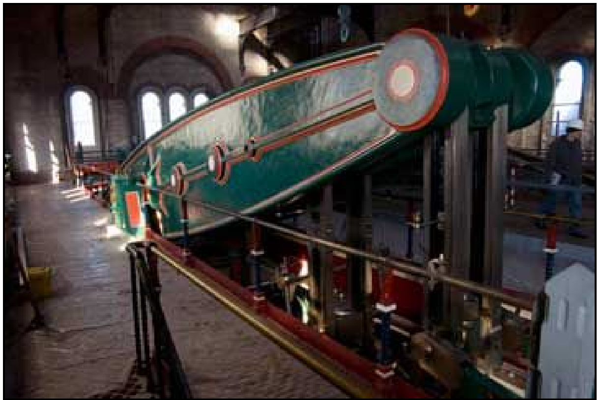
Each beam engine had 52 ton flywheels and 47 ton beams
