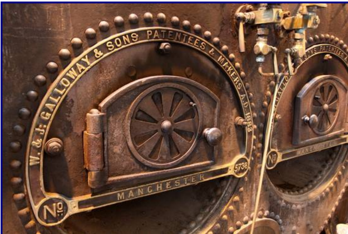
A coal-fired Galloway steam boiler dating from about 1883
