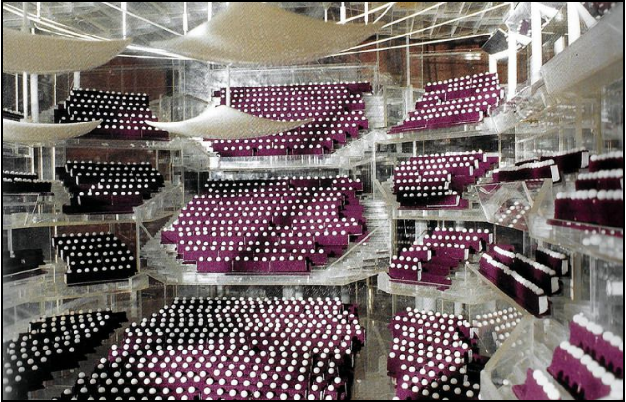
Scale acoustic model of Manchester Concert Hall, Arup Associates
