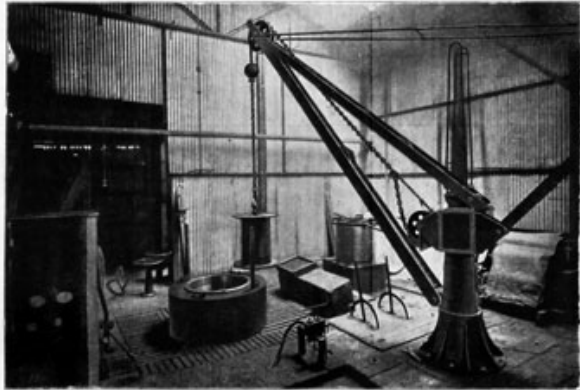
TANK FOR TESTING GUTTA PERCHA CORES HYDRAULICALL.
