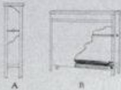
A—End view of Trane Heat Cabinet (inside view), showing position of the damper.
