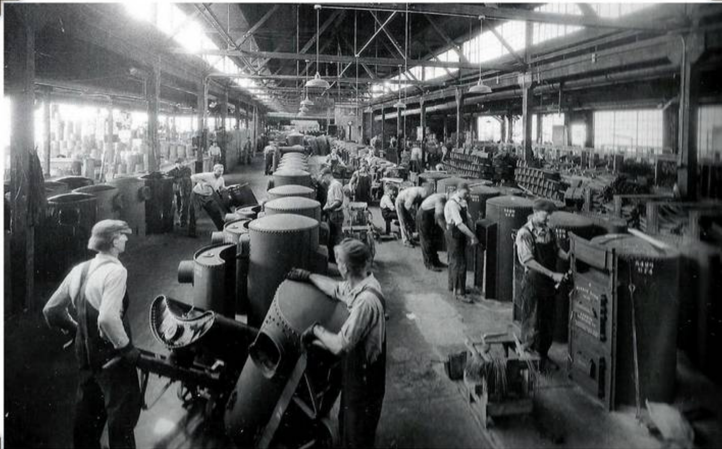
Assembling "Torrid Zone" furnaces The Lennox Furnace Co, Marshalltown, Iowa, 1930's
