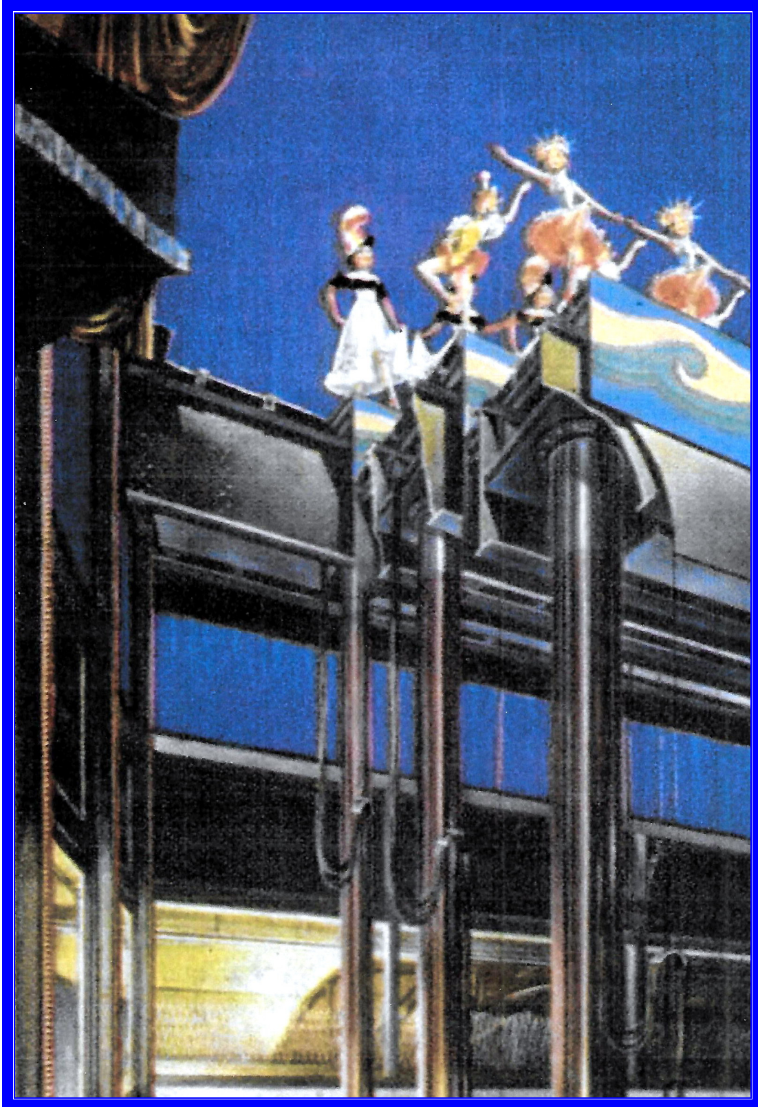
Cut-Away Drawing of the Stage Elevators lifting performers
