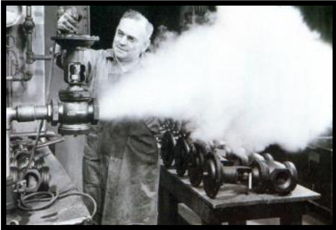
Testing a steam control valve at the Johnson Factory, 1944.
