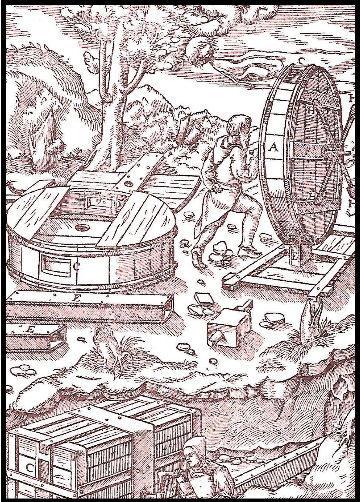
Hand-operated fans for mine ventilation, Germany, 1556.
