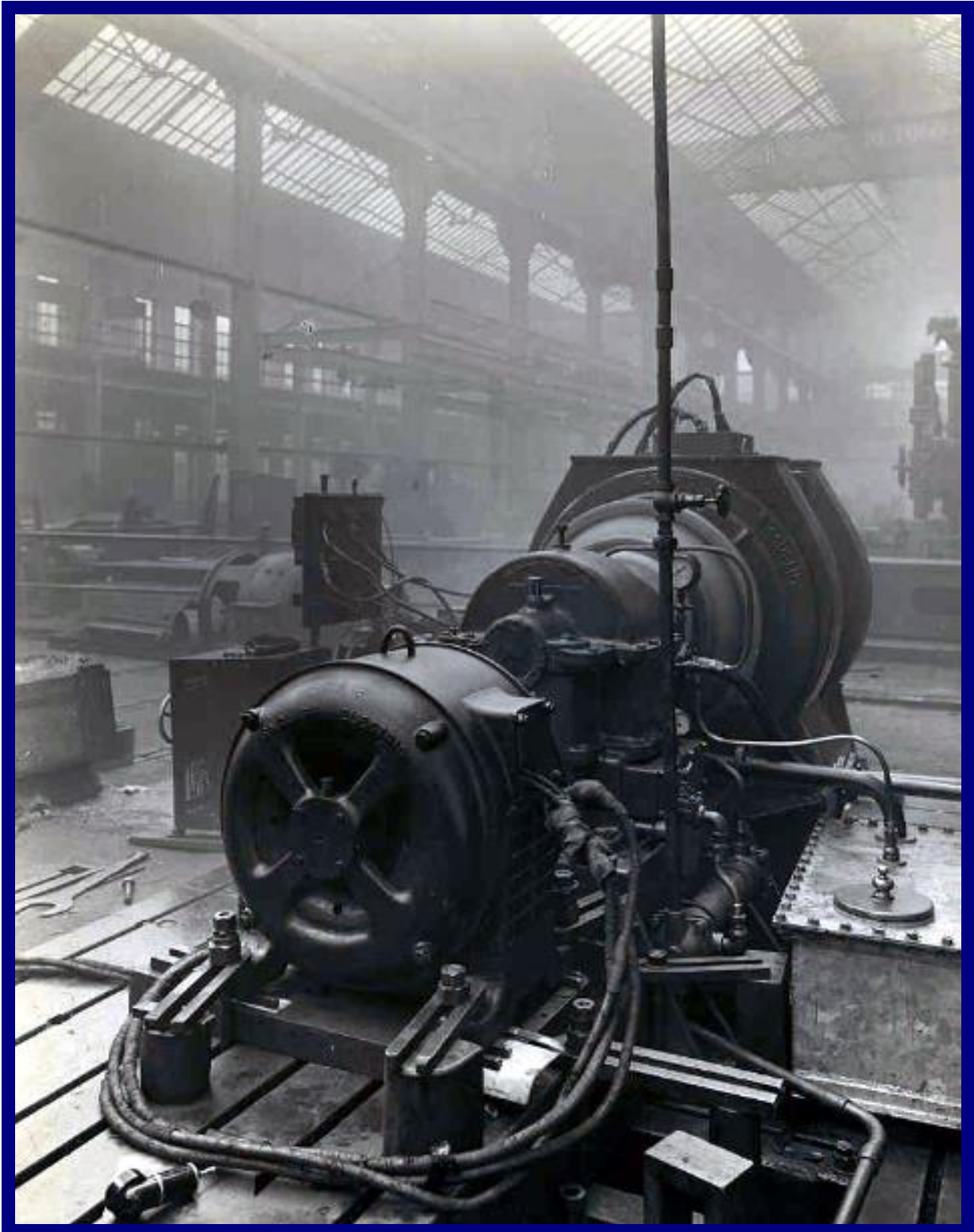
Centrifugal compressor and motor on test at English Electric, early 1930s.
