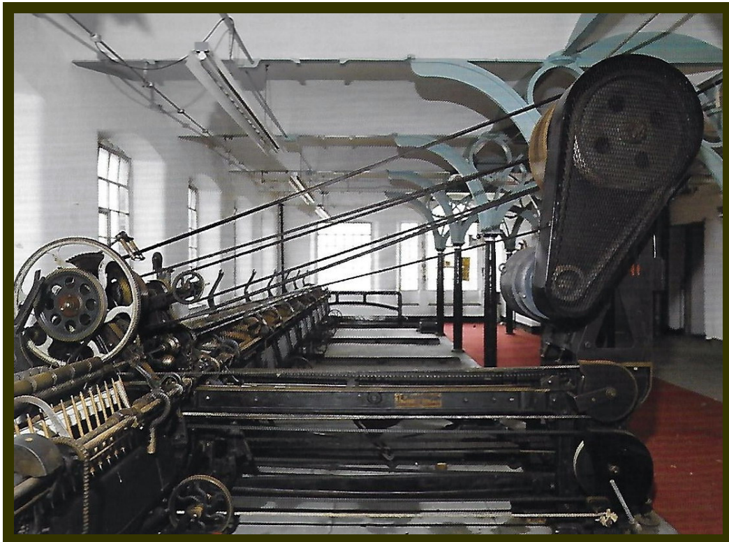
A later self-acting very long Spinning Mule at Stanley Mill (photo of 1910).
