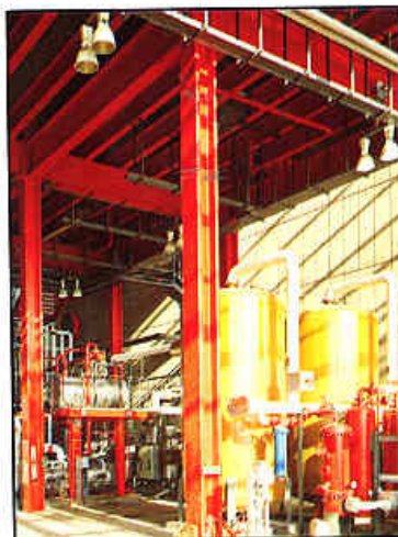
Opposite Page Historic skills applied to new processes, in this case penicillin production. The twin stacks are part of the solvent recovery plant
