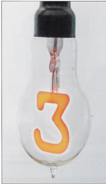
1922-1925 OSGLIM, G.E.C., London. Neon indicator. Used in cinemas and theatres to indicate seat locations, room numbers etc. BC 240v 5w 2¼" x 4¼"
