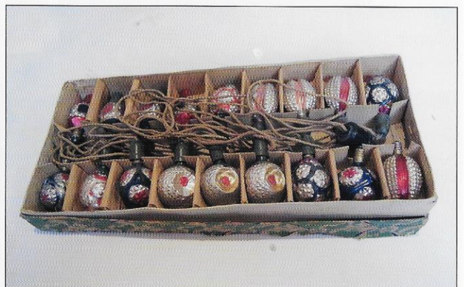
1930s INSIDE SILVERED LAMP SET NO. 3701'. 'Foreign' make. 16 lamps and 2 spares. Moulded in clear glass, Internal silver coating, externally hand painted. Notoriously unreliable due to internal overheating in use. V.I.R. flex. Series wiring to Bakelite BC adaptor. 16v bulbs. 240v circuit (open circuit) 14" x 6" x 2"
