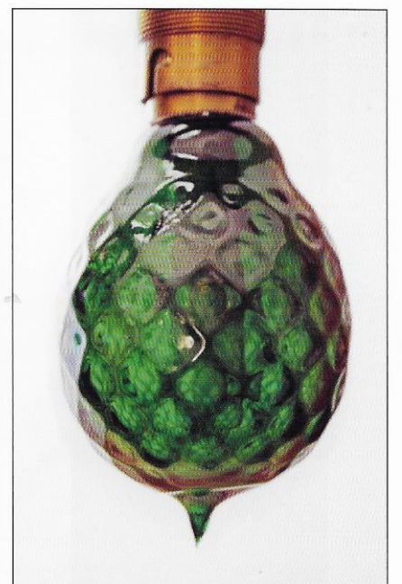
1886-1893 'THE EDISON SWAN'; Edison & Swan United, England. "Fancy Lamp". Diamond design moulded in glass. The bulb has been opened and tubular carbon filament lamp inserted. Original brass tubing bayonet cap retained, Plaster of Paris insulation and arc contacts restored. Rating N/A. 2 1/3" x 4" (Pages 33 & 205)
