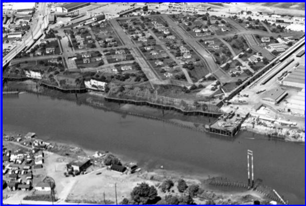
During WWII, the giant roof of the Boeing Aircraft Factory was camouflaged as a housing estate.
