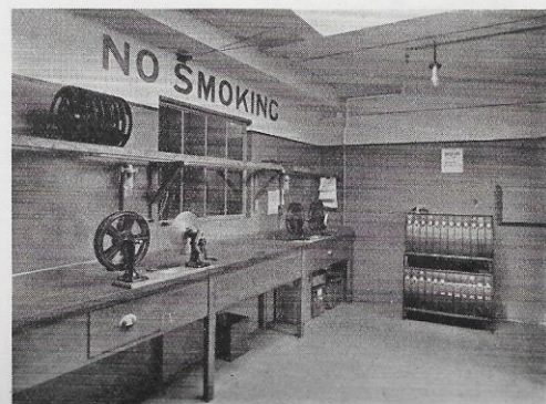
In the rewind room it is still found expedient to rewind films by hand. This is curious in view of the striking advances made in the projector machines.
