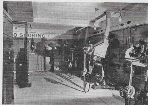
The projection room must be of sufficient size to accommodate at least two machines and should be planned on the centre axis of the cinema. On the left of the photograph is the talkie apparatus.
