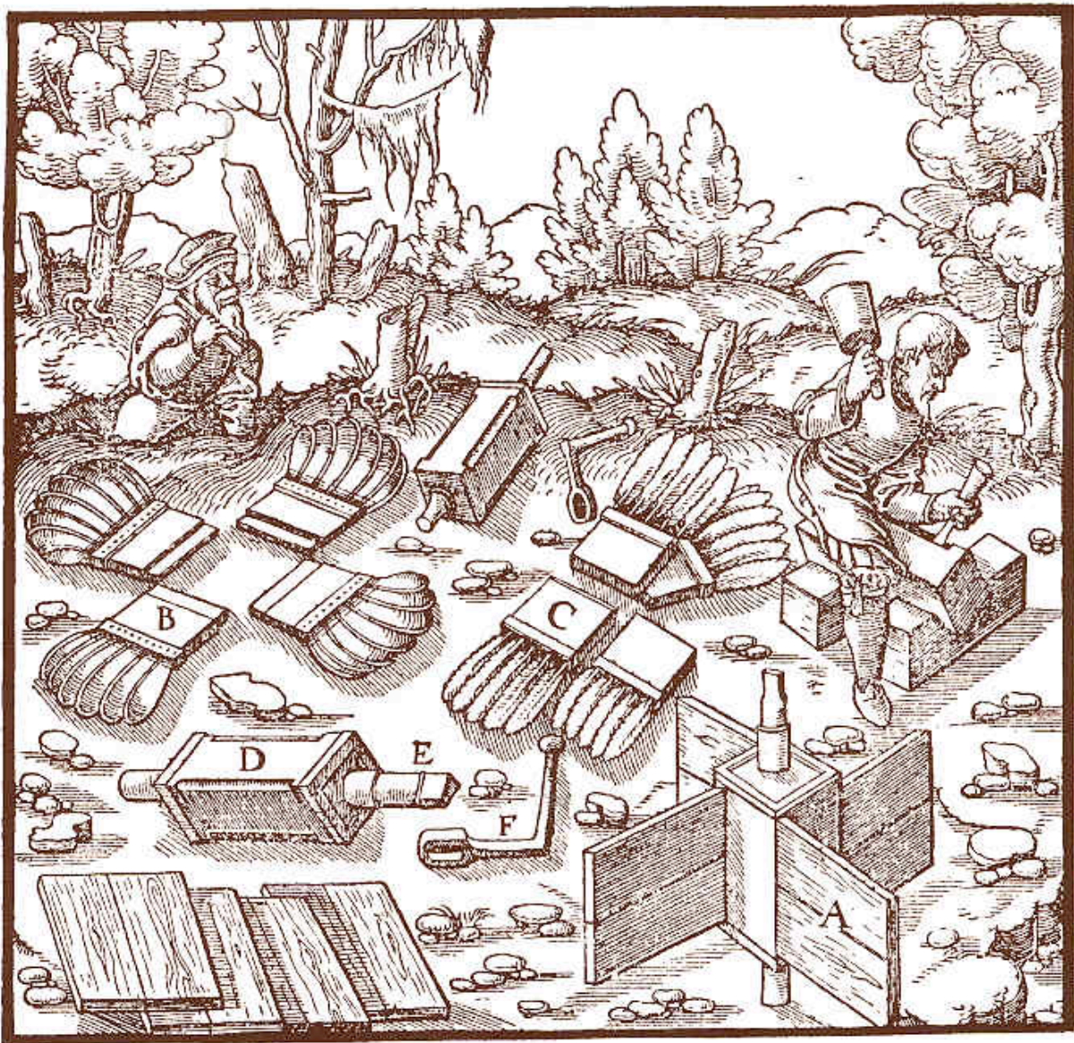
2. Woodcut: Making Fans for Mine Ventilation. Notice the fan blades tipped with goose feathers. ( De Re Metallica , Georgius Agricola, 1556). DRM: Book VI, p207
