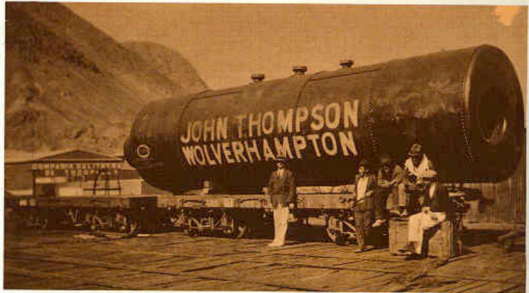
A John Thompson Dishended Lancashire Boiler arriving in Tocopilla, Chile, South America
