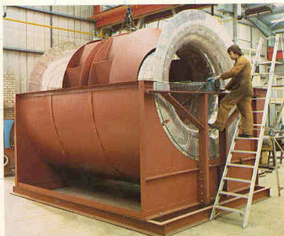
A large high efficiency variable speed V-Aerofoil Centrifugal Fan for application on test with temperature down to -40°
