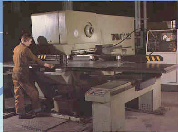
An N.C. nibbling machine producing A.H.U. frames prior to forming.
