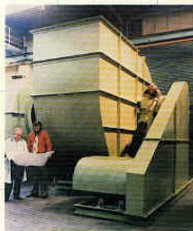
One of three large V. Aerofoil High Efficiency fans supplied for the Shell/Esso Brent 'B' Condeep drilling platform.
