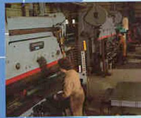
A.H.U. panels being formed.
