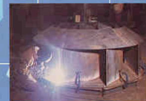
Welding a 2.5 m fan impeller. Low temperature application (-40°C)
