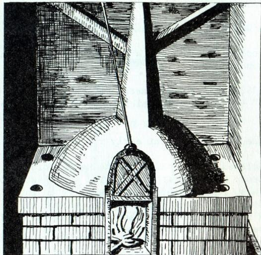
Fig. 4.4. Böckler's stove, with warm-air ducts
