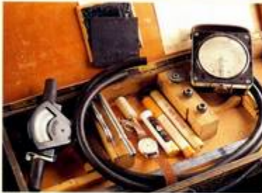
Part of the survey equipment used by Rudi Kohner in the 1940s. On the left is the Filometer made by Metrovick which measures the pressure drop across air filters. The square instrument on the right is the Poole Airmeter, made by Oldham & Sons Ltd, for measuring air velocity.
