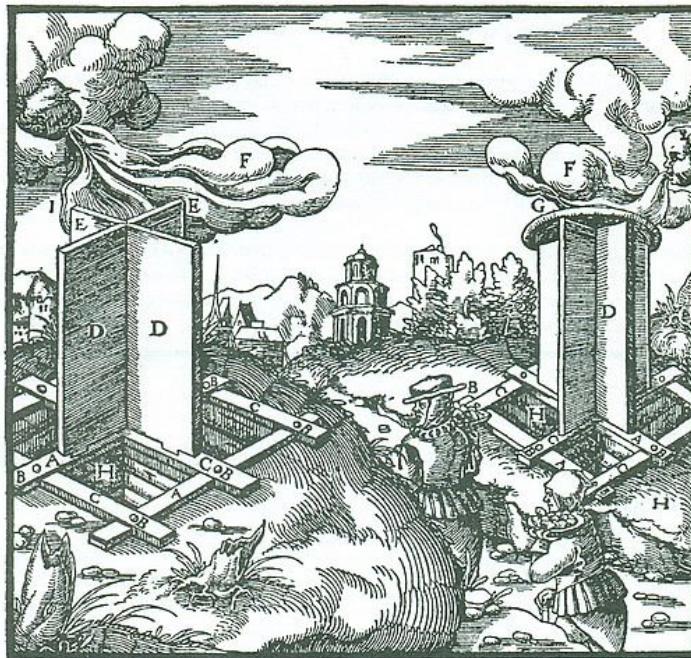
Woodcut: Ventilating Machines (Wind Collectors) for Mines, Germany. De Re Metallica, Georgius Agricola [51], 1556. From 13, p. 201.
