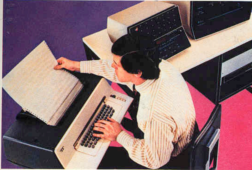
The JC/80, introduced in 1972, is the first mini-computer designed and fully standardized to meet building control criteria.
