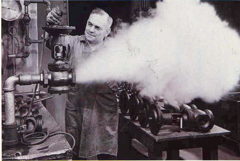
Control valves are tested before leaving the factory in 1944.
