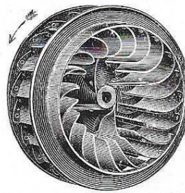
Loose blades, showing blades' form and proportions.
