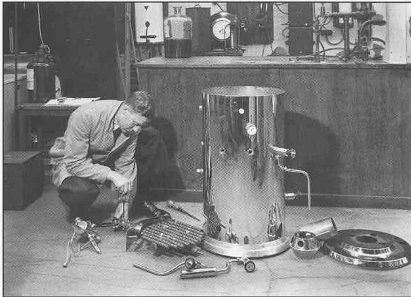
116. Efficiency Test on a Cafe Boiler, Water Heating Laboratory, Watson House, Fulham, probably early 1970s. North Thames Gas Board. (RFH, neg.729-1).
