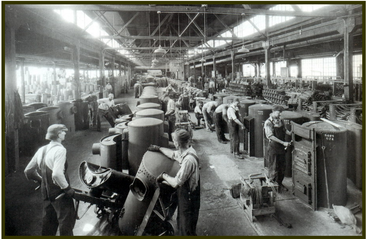
Assembly of Torrid Zone heating furnaces, 1930's "Lennox: The First Hundred Years 1895-1995", 1995 (CIBSE Heritage Group Collection)
