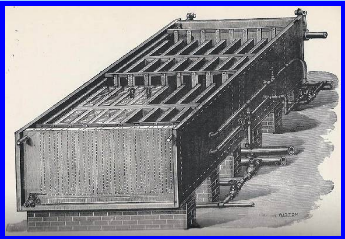
Ice-making tank using the plate system by Pontifex and Wood
