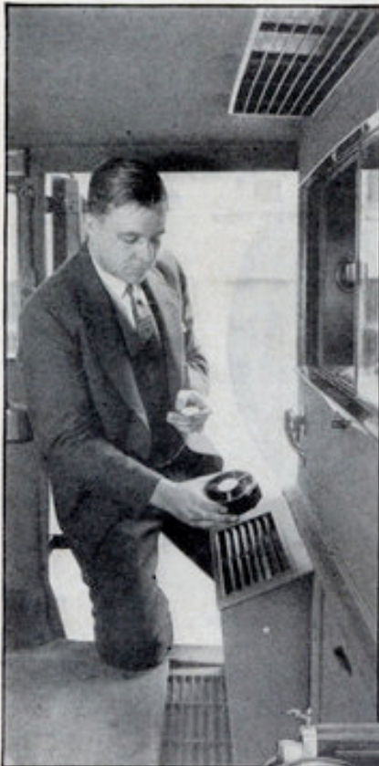
Through the grills seen above, fresh air enters and old air is expelled in the first air-conditioned car seen at right
