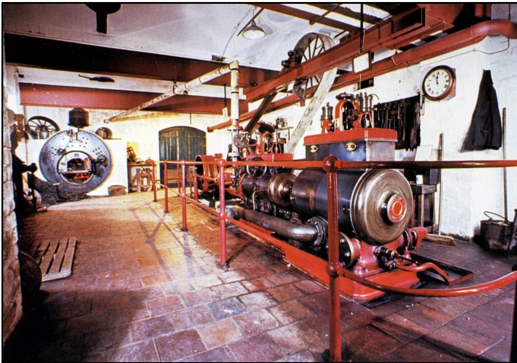
Marshall Reciprocating Steam Engine and Boiler
