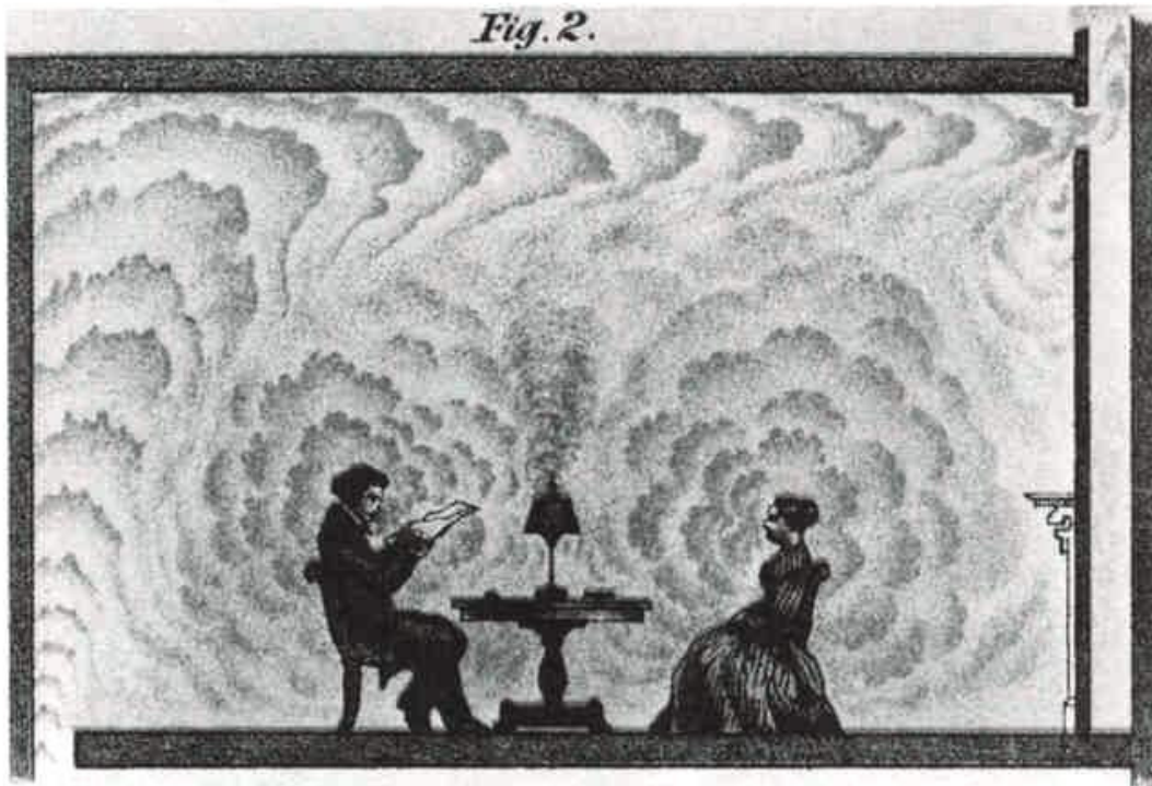
Fig. 10.14 Fresh, heated air, admitted at lower left, rises and flows across ceiling to the exhaust register at upper right. The clouds of heavily vitiated air, purple and unpleasant, which surround the man and woman, are nearly undisturbed by the badly designed heating system. Lewis W. Leeds, Treatise on Ventilation (New York, 1871) fig. 2.
