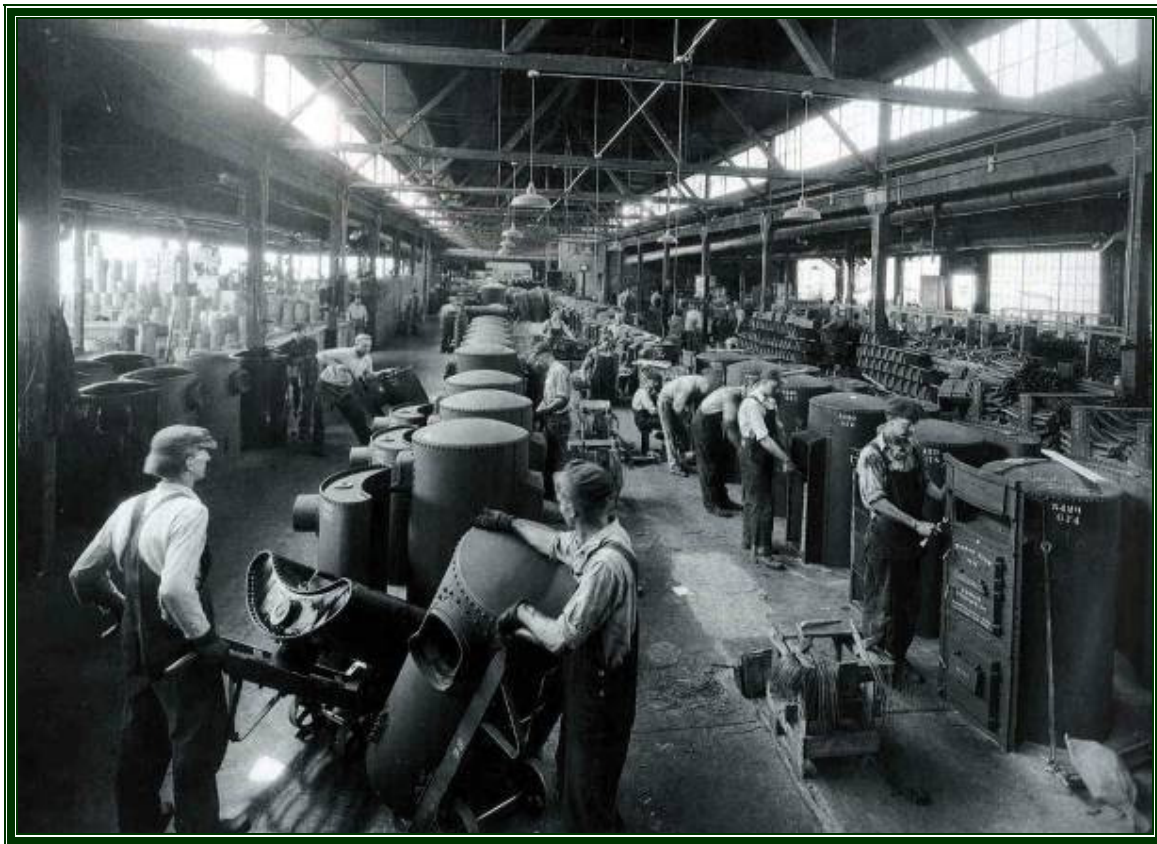
Assembling "Torrid-Zone" Furnaces during the 1930's
