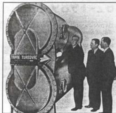
Reuben Trane's company developed a centrifugal compressor with a hermetically sealed motor in 1938. The technology fueled the development of machines to supply chilled water to air condition large buildings.
